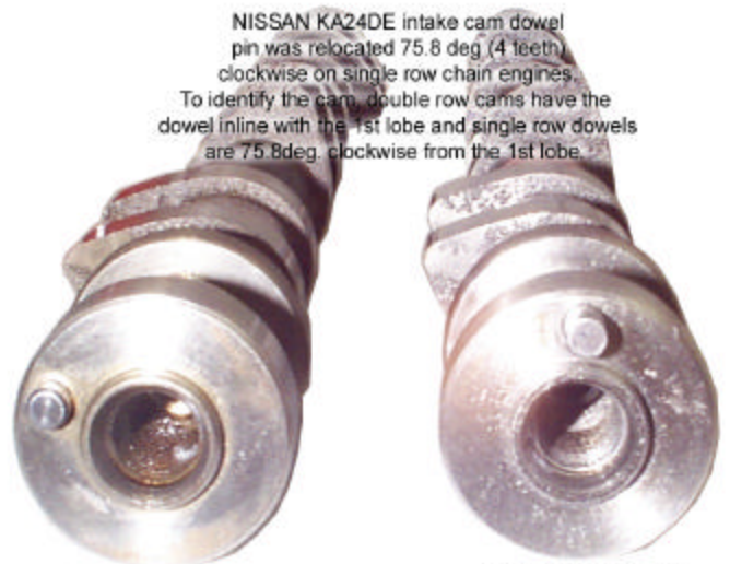
DOUBLE ROW CHAIN TYPE INTAKE CAM
