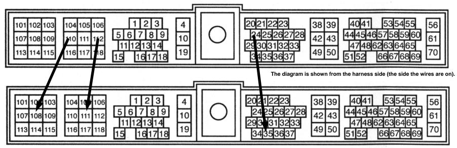
The <u>rear</u> O2 sensor must be changed to a EARLY 3 WIRE type sensor or the MIL light will come on. Transfer the plastic electrical plug from the original 4 WIRE sensor to the new EARLY 3 WIRE sensor using the diagram numbers.
