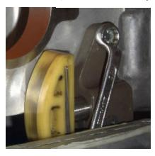
The upper tensioner bolt is difficult to unbolt, but it can be removed using a **10m.m. deep offset box wrench** (Snapon or Sears). You can't see the upper chain tensioner bolt with the front cover installed, but this is how it looks with the offset wrench on it. Back it out as far as possible with the wrench, then use 2 long screwdrivers on the bolt head to twist it out the rest of the way. Remove the tensioner.
