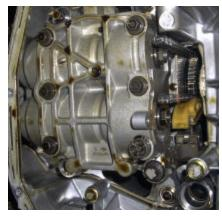
Remove the oil pan and oil pickup. Unbolt the chain guide. The lower tensioner/guide bolt will hit the cover just before it falls out, so it must be pried on slightly or cut to remove it. Remove the chain guide covering the sprocket and unbolt and remove the sprocket. The drive chain can then be cut using bolt cutters and remo ved . Any other method of cutting the chain may cause metal chips to enter the engine. Remove the chain tensioner (see next step).
