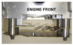
The stack up should look like this if the plates are installed correctly. Inspect your work carefully. Install the oil pan using suitable silicone sealant. An additional quart of oil capacity is created by removal of the balancer assembly, so check the oil level carefully.
