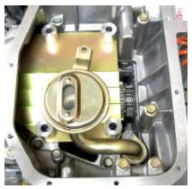
Install the oil scraper plate and reinstall the oil pickup (it's hard to tighten if done later). Glue the **long** spacers to the oil scraper as shown above. You may need help holding all of this in place until the long bolts are in place in the next step.
