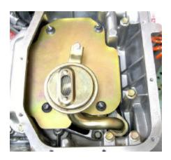
Install the oil baffle plate using the 4 original assembly bolts. Torque all 4 bolts first to 37 lb/ft. Finally turn each bolt an additional 90 degree. Bolt the oil pickup support bracket to the oil baffle using Locktite and the supplied bolt, washer, and aluminum spacer.
