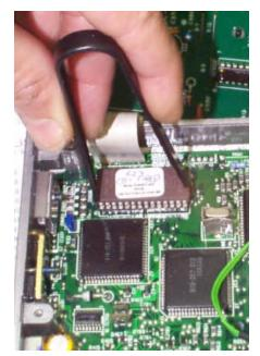
REMOVE THE CHIP USING A RE-MOVAL TOOL. TRY RADIO SHACK IF YOU DON'T HAVE ONE.
