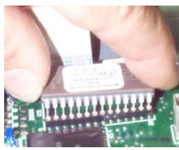
INSERT THE FRONT ROW OF PINS AND PUSH CHIP FULLY INTO THE SOCKET. INSPECT THAT ALL PINS ARE IN THEIR SOCKETS.
