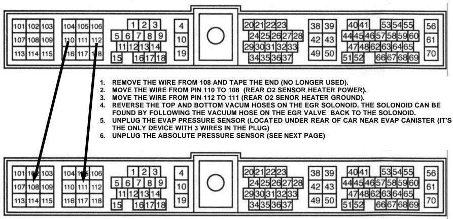
The <u>rear</u> O2 sensor must be changed to a EARLY 3 WIRE type sensor or the MIL light will come on. Transfer the plastic electrical plug from the original 4 WIRE sensor to the new EARLY 3 WIRE sensor using the diagram numbers.
