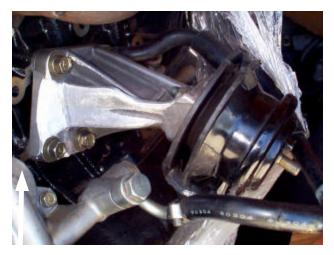
If you are installing the turbos with the engine in the car, modify the motor mount support rear web as shown. This will allow enough room to clear the 4 turbo mounting studs.
