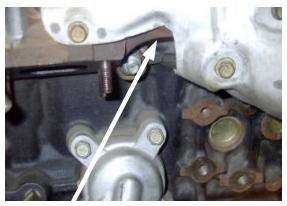
Notch the right side manifold heat shield as shown to clear the compressor housing.
