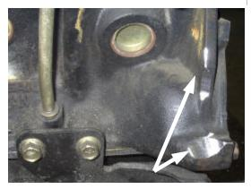
Grind the engine block as show on the left side to clear the turbo housing. Also check that the dipstick tube does not touch on the compressor housing. Bend the dipstick tube as needed.
