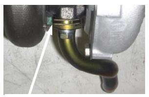
Install the supplied oil drain spacer as shown on the left side oil return tube to clear the compressor housing.
