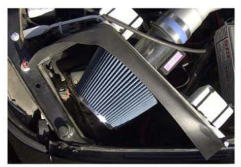
EXAMPLE OF A COLD AIR BOX ON A NX2000 RALLYE CAR Note that the aluminum sheet metal is supported only by a 1"x.250" aluminum support bracket. The sheet metal is edged on all sided with special weather stripping to seal out heat and allow wiring and hoses to pass around it without interferance.
